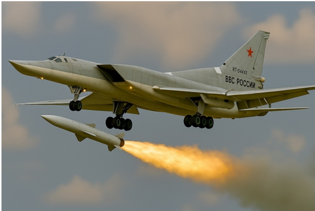
Figure 18 - A Russian Tupolev Tu-22M3 strategic bomber releases a Kh-22 air to surface missile.
