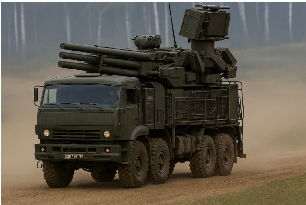
Figure 16 - The Pantsir-S air defence system, frequently used for short range air defence.
