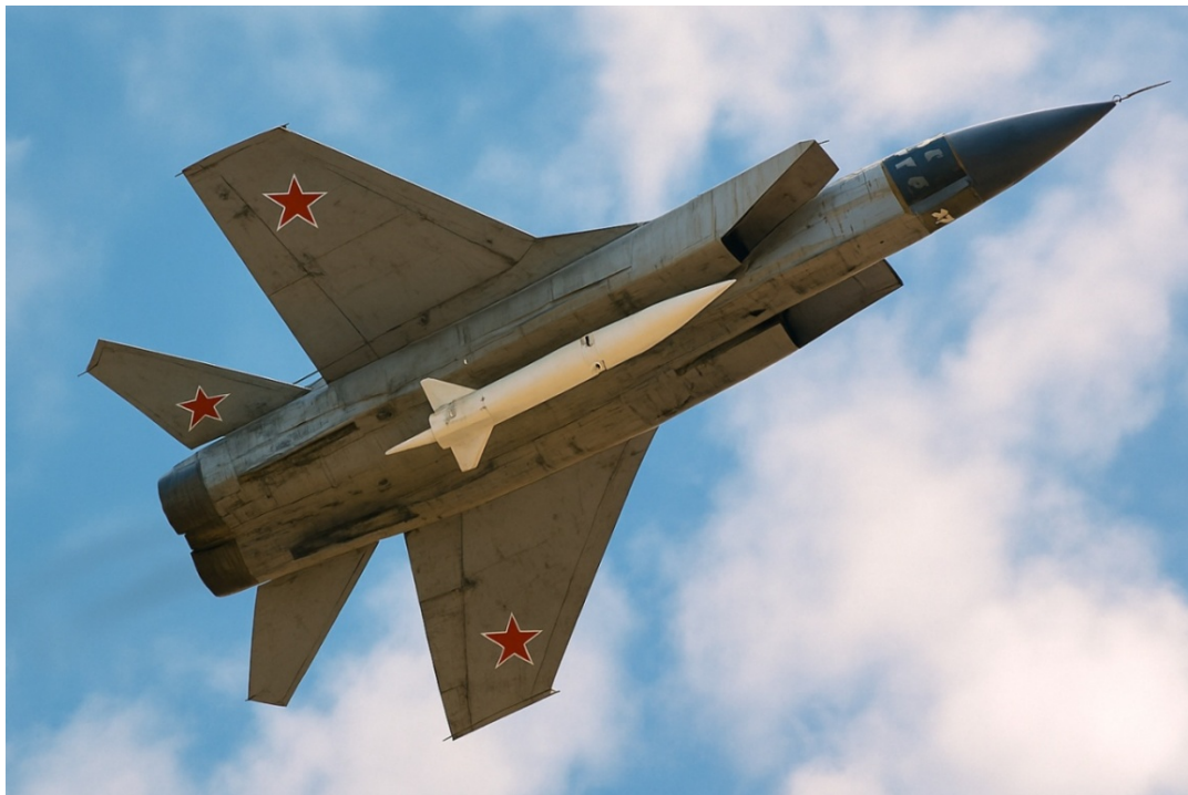
Figure 19 - A MIG-31K, configured for the transport and release of the Kh-47M2 Kinzhal hypersonic ballistic missile.
