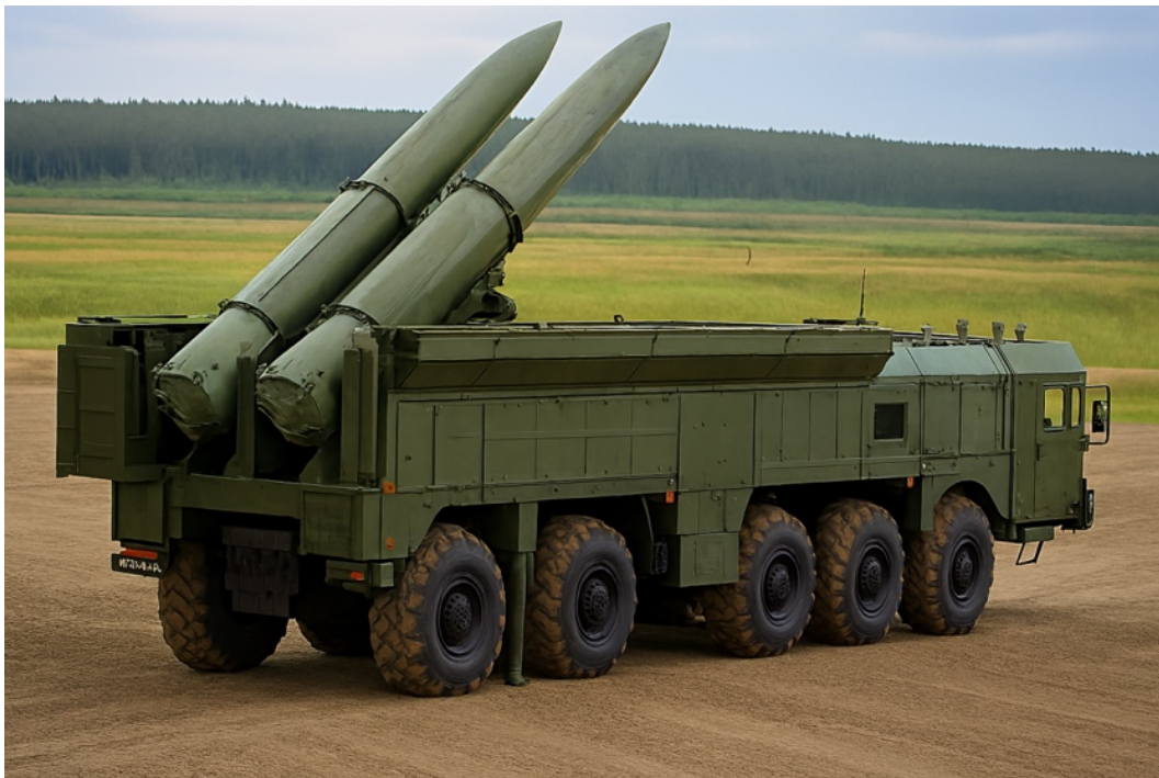
Figure 11 - An Iskander-M TEL in firing position.
