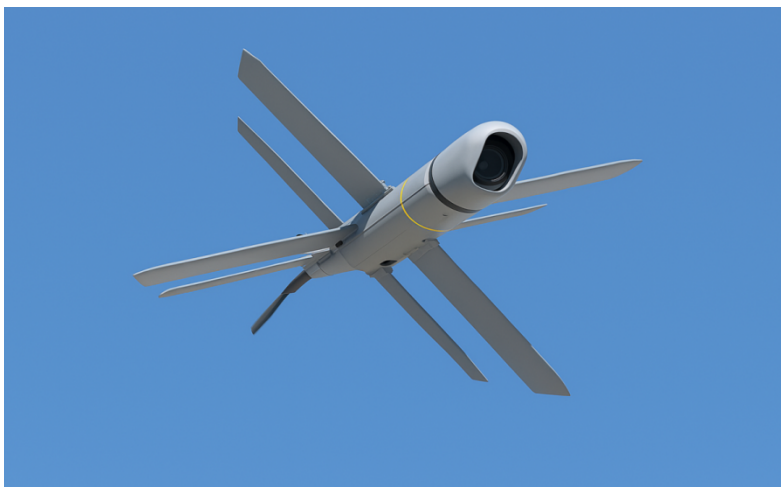
Figure 13 – A Lancet-3 loitering munition flying towards the target.
