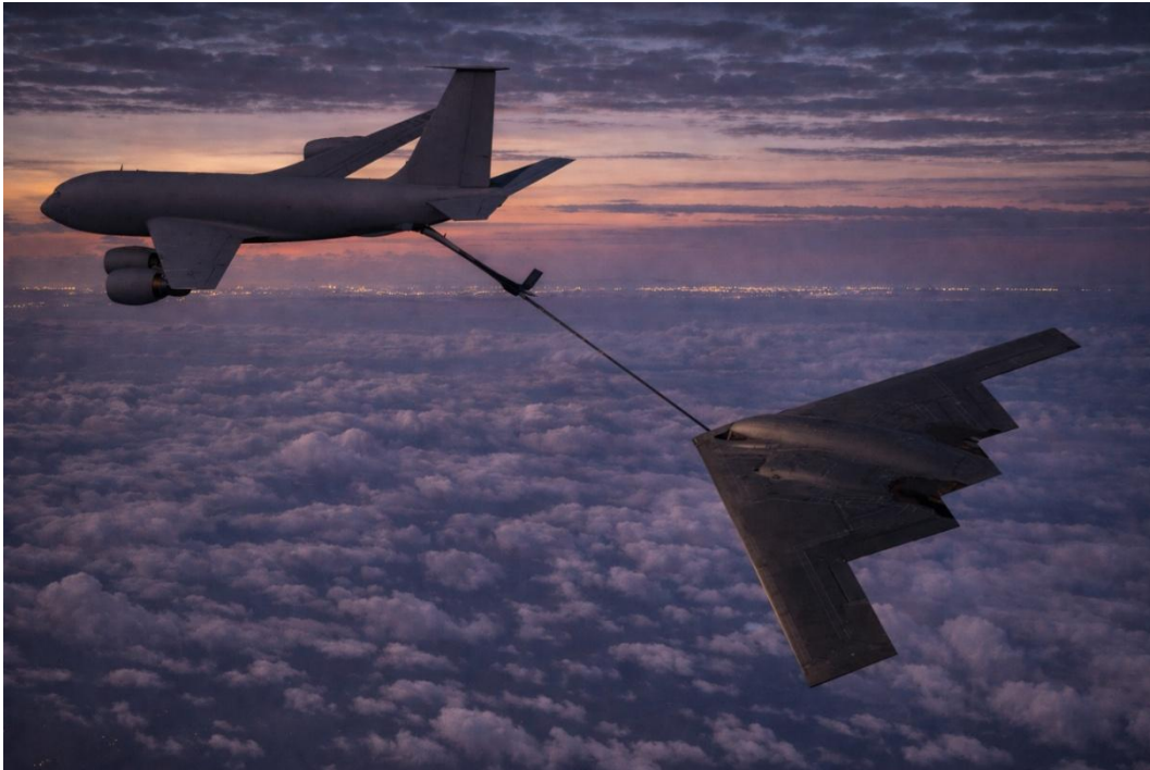
Figure 2 – A B-2 Spirit bomber engaged in aerial refueling with a KC-135 Stratotanker.
