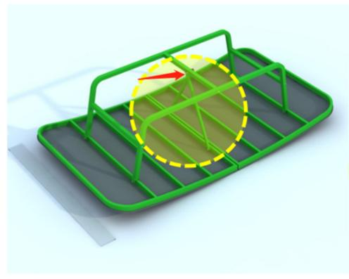
Connecting U Legs and Top A and Top B with Fix Table Tube AB Use 8\*120mm and 8\*100mm Screws and Bolts.
